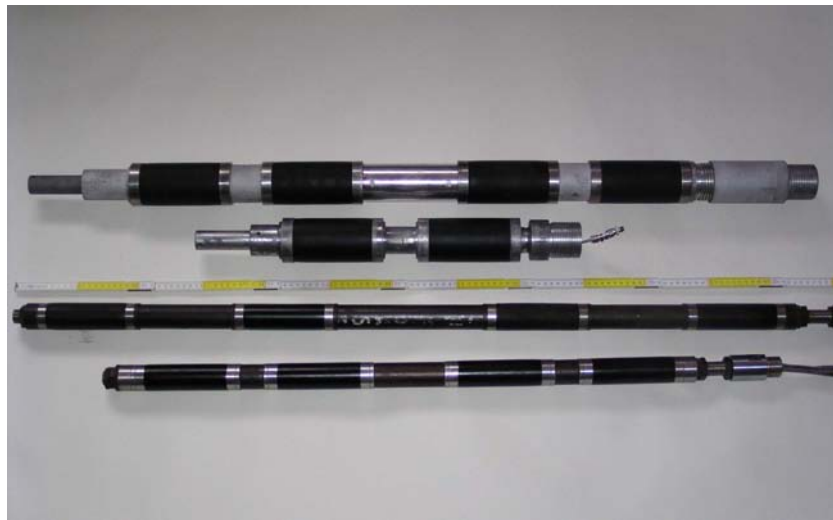
Figure 8 Selection of packer equipment with diameters of 42 mm and 70 mm
