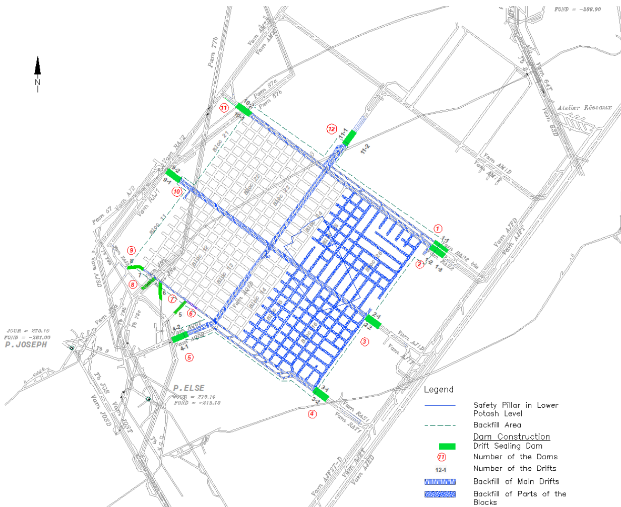
Figure 5 Overview of the Location of the Planned Dams Sites as well as the Main Drifts and Voids to be Backfilled in the Storage Blocks
