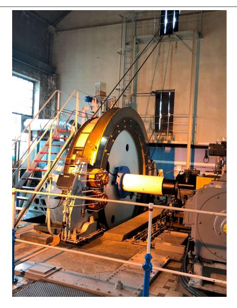
The extraction machine features a cage and a counterweight.
