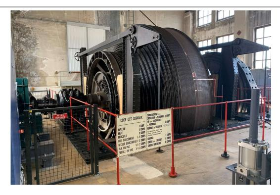
The extraction machine uses two opposing cages. The characteristics are as follows:
